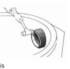
Decide which size collar is appropriate for the connecting pipe. Cut away the surplus part of the coupling using a knife. A special recess is provided for this purpose.
