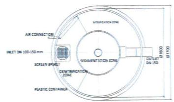
note: Drawing of WWTP for backfill or concreting. Assembly make according to the instruction for installation.
