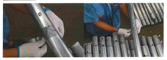
Please use the tape wrapped around the gap between the steel skeleton after installing.
