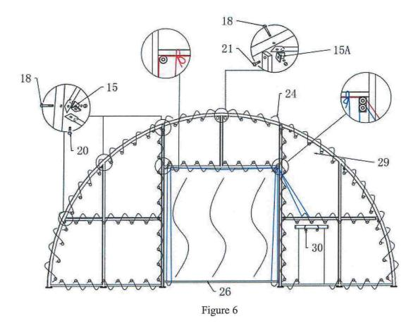
1.Please install the front and back door frame and cover as above figure 6 shown.Find corresponding bolts and tubes,connect each other then knit rope(No.24) on front and back cover (No.29) to lace the grommet on the tubes evenly.
