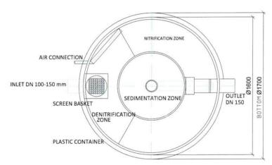
Note: Drawing of WWTP for backfill or concreeting. Assembly make according to the Instruction for installation. \* In case the WWTP has to be instaled deeper than maximal allowed dimension (see the drawing) or the soil load around the WWTP or underground water level i higher then we strongly recommend statically secure the WWTP tank (e.g. concreeting).
